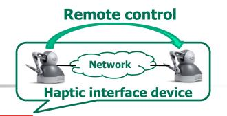
Remote control system with haptics in which a user can remotely operate a haptic interface device by using another haptic interface device while watching video
