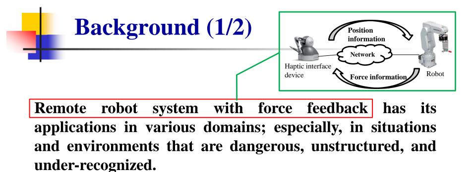
Through a haptic interface device, a user of a system can remotely operate a robot with a force sensor while watching the video.
