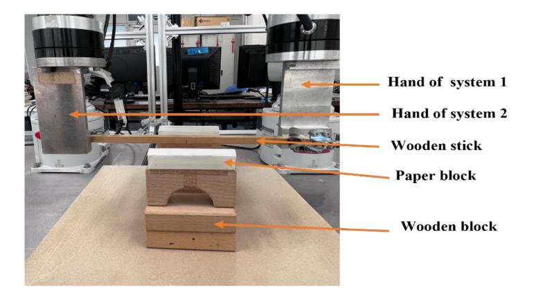
The task was to touch each paper front and back with the wooden stick by using the haptic interface device.
