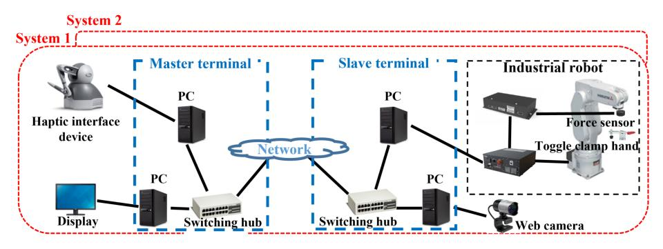
**Configuration of two remote robot systems with force feedback**
